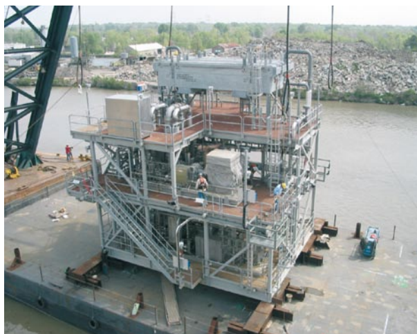
Figure 5. Oil free screw gas compressor for vapour recovery service on offshore platform.
